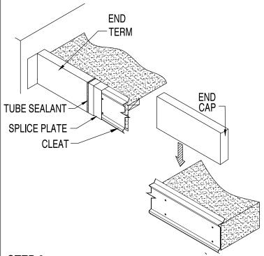
**STEP 3** : Installing Fascia Cover End Caps and End Terms Apply a bead of Tube Sealant inside End Cap or End Term and place a Splice Plate under each end of the End Cap or End Term. Install the Fascia Cover End Caps and End Terms by hooking the drip of the Fascia Cover End Cap or Term onto the roof side kick up of the Cleat and push down onto the lower kick out of the Cleat.
